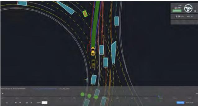
First, CEP (Continuous Evaluation Platform) is a high performing distributed system that runs large scale simulation tasks. This system supports many types of workflow, like simulation, SIL tests and model benchmarking. CEP has a dedicated web UI where every engineer can easily submit a ticket to run their tests.
