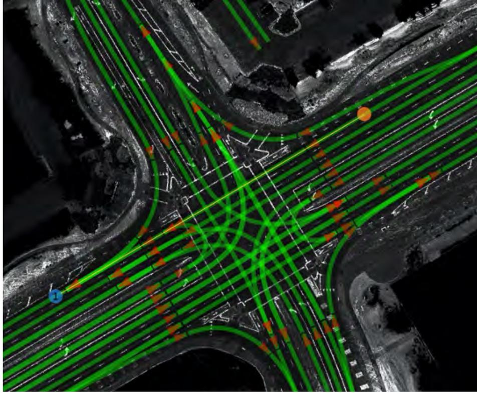
HD-Maps comprise comprehensive information about the world that is pertinent to our autonomous vehicles. We have in-house technologies to build HD-Maps with centimeter-level precision, detailed and accurate 3D geometric structures, as well as rich semantics including lane, traffic control information, etc. We have built maps covering thousands of kilometers in our test areas.
