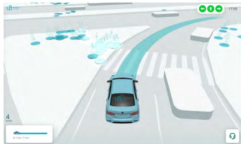
▲ A call for help button is located at the bottom right corner of the passenger visualizer
